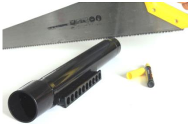
Figure 58: Cutting the TufMan™ Manifold
