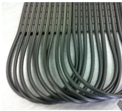
Figure 71: Standard method of flipping and looping the Collector
