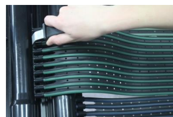
Figure 66: Using Pointy Nosed Pliers to peel the Collectors Webbing
